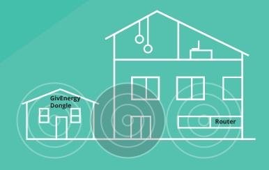
When installing the Inverter into an outbuilding, such as a garage, the signal may not be strong enough to reach the dongle.
