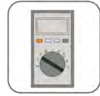
Multimeter ≥ 1000V DC
