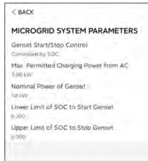
figure 8-42 MicroGrid System Parameters
