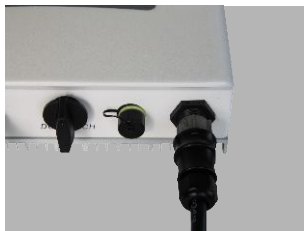
▲ Figure 4.16 Connect the AC Connector to the Inverter
