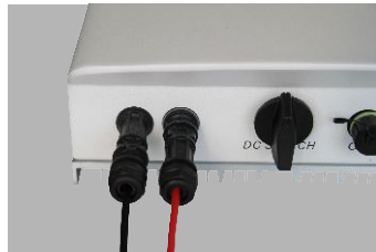
▲ Figure 4.10 Connect the DC Connectors to the Inverter
