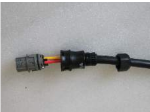
Figure 4.16 Connect Wires to the Terminal
