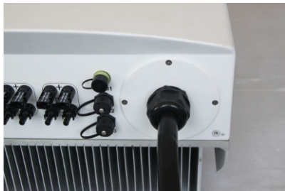
▲ Figure 5.18 Tighten the AC terminal
