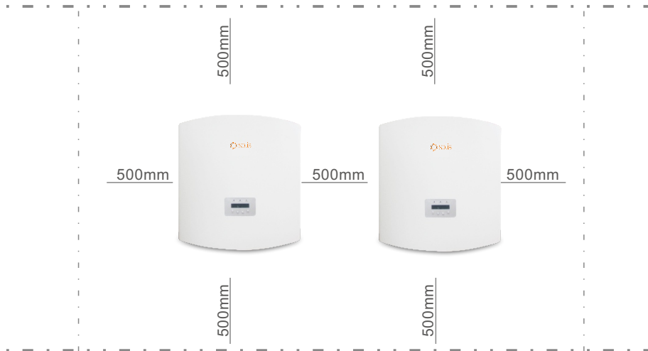
▲ Figure 5.2 Inverter mounting clearance
