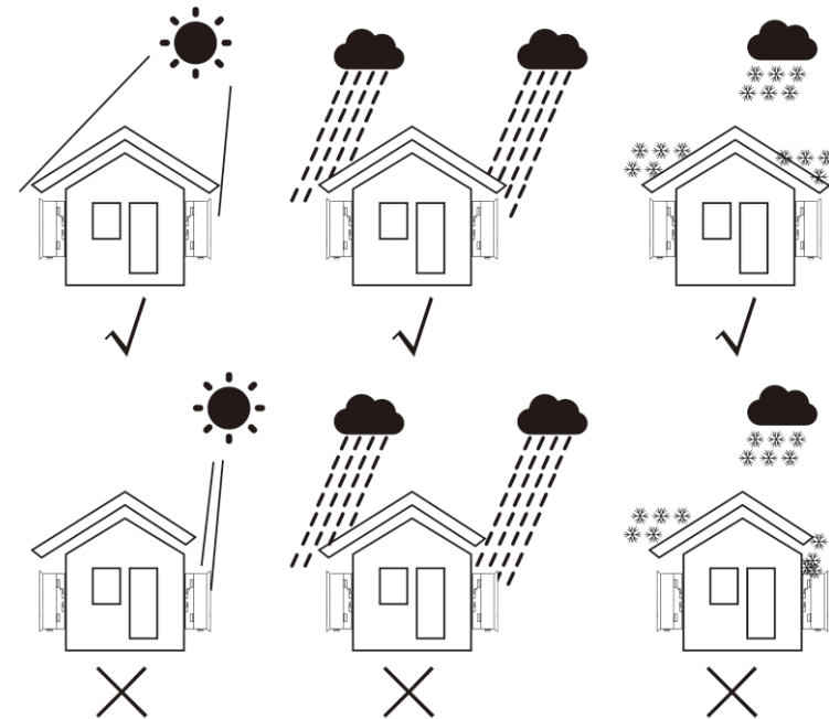
▲ Figure 5.1 Recommended installation position
