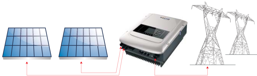
Figure2-1 PV Grid-tied System
