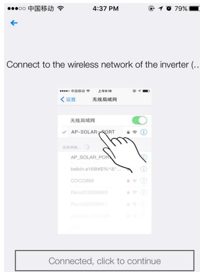
Please connect your mobile phone to the network of the WiFi monitoring device, the network names consists of AP and device SN.
