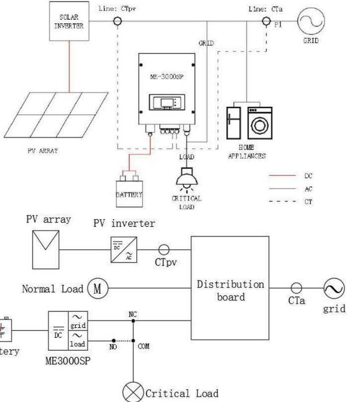
**Step 1:** Location of CTa: L wire of incoming mains. Location of CTpv: L wire of PV inverter's output.
