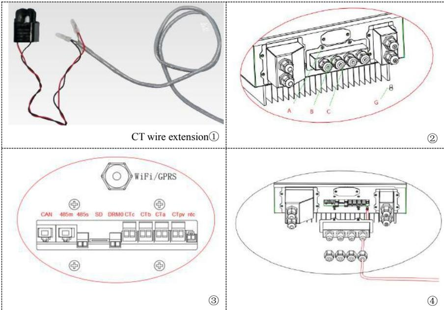
**Step 3:** Loosen 4 screws(part A)using a screwdriver(fig.4-7②)
