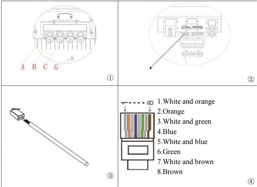
The logic interface pin definitions and circuit connections are as follows:
