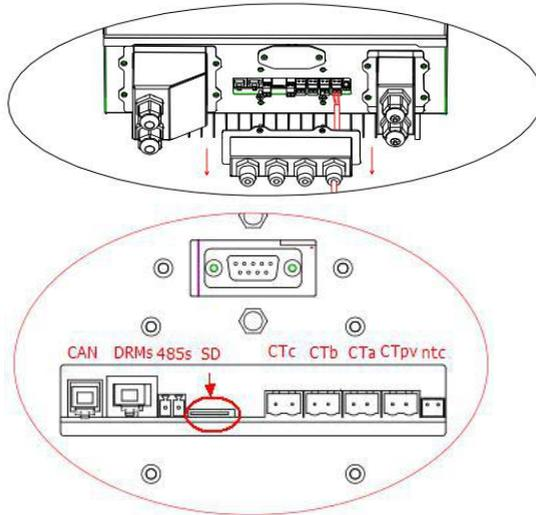
**Step 2** Press the SD card and take it out.Insert the SD card into a micro-SD card reader,then insert micro-SD card reader into a PC;(NOTE:micro-SD card reader&PC are not provided by SOFARSOLAR).
