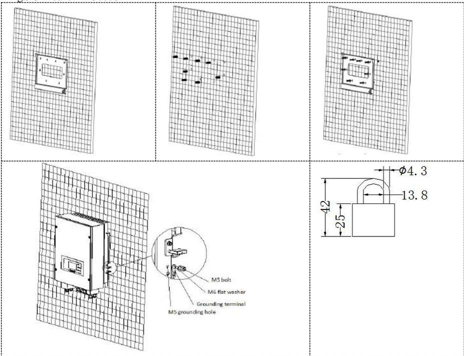
Step 1: Put the mounting bracket properly on the wall, mark these 8 drill holes using a marker pen. Drill 8 holes (drill bit 6mm) on the wall.
