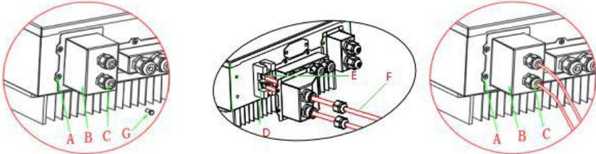
Step 1: Loosen 4 screws(A) using a screwdriver(Fig.4-2);
