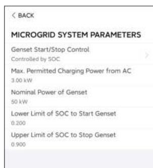
figure 8-42 MicroGrid System Parameters
