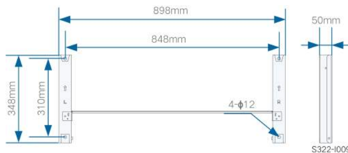
figure 4-1 Dimensions of Mounting-bracket
