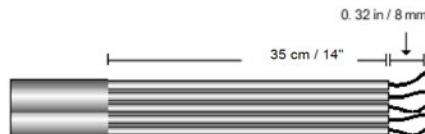
Figure 33: Insulation stripping – AC
