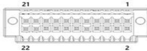
Figure 4: Industrial connector layout
