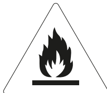
Caution: Risk of fire/ flammable materials
