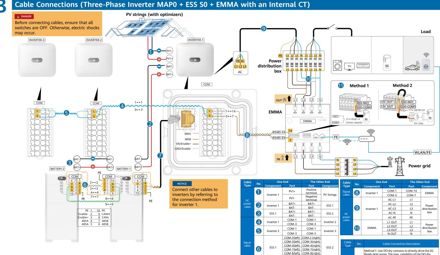
Signal cables must be outdoor shielded twisted pair cables.
