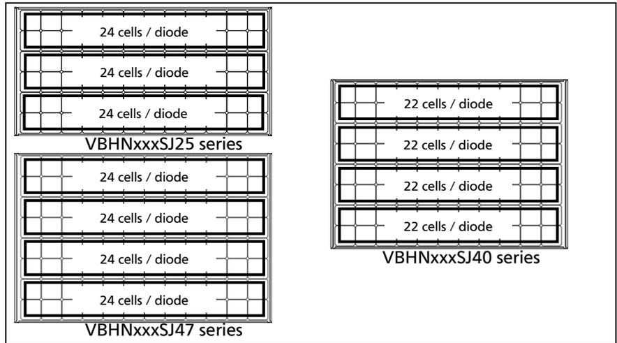
Figure 4: Number of series cells per bypass
