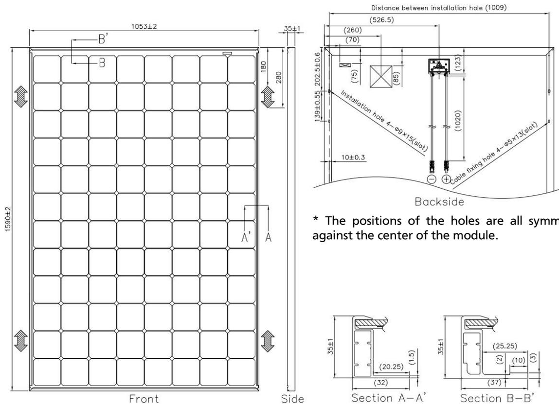
\* The positions of the holes are all symmetry against the center of the module.
