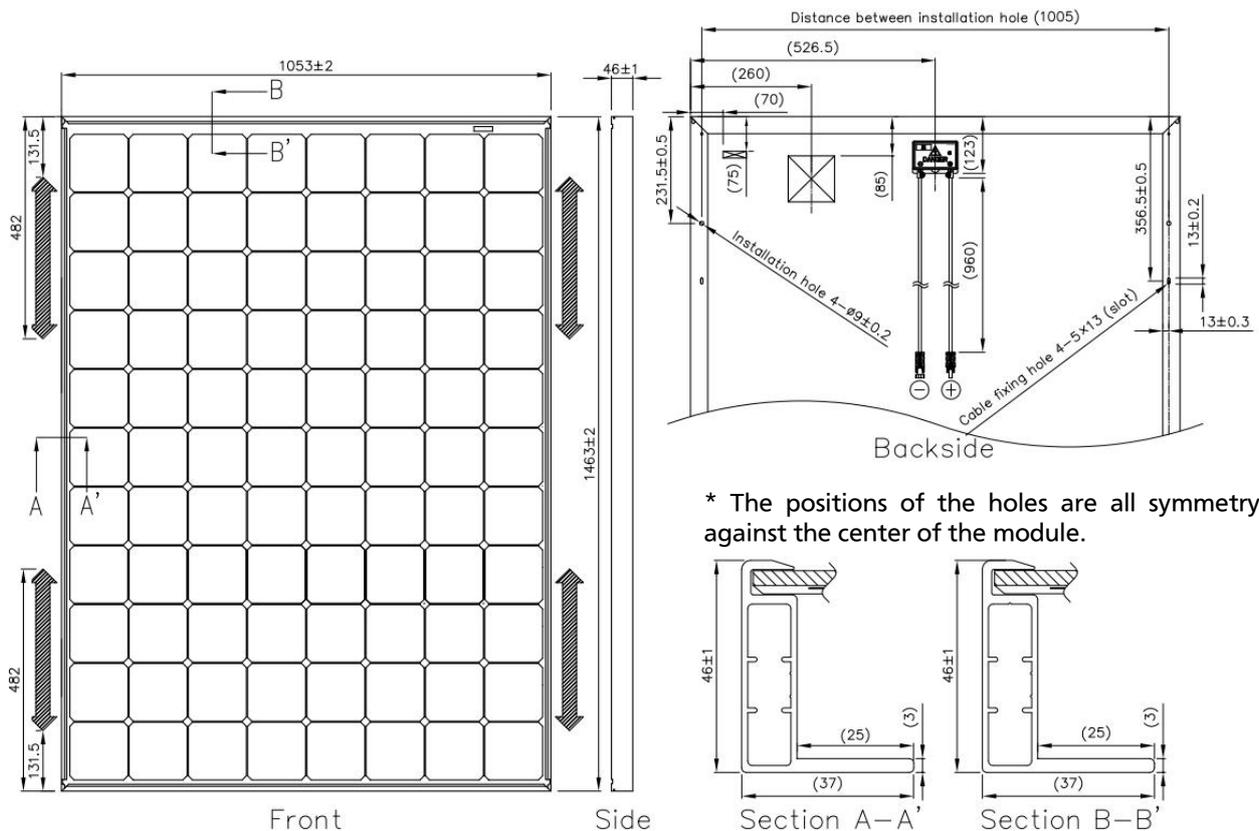
Note) A module is installed using 4 points, symmetrical mounting within setting range (shaded).
