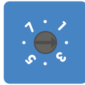
Rotary switch set to position 2
