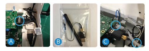
**Ethernet:** For ethernet connections to broadband the Wifi dongle should be removed from the Pi and put in the labeled plastic bag and secured it safely inside the unit:
