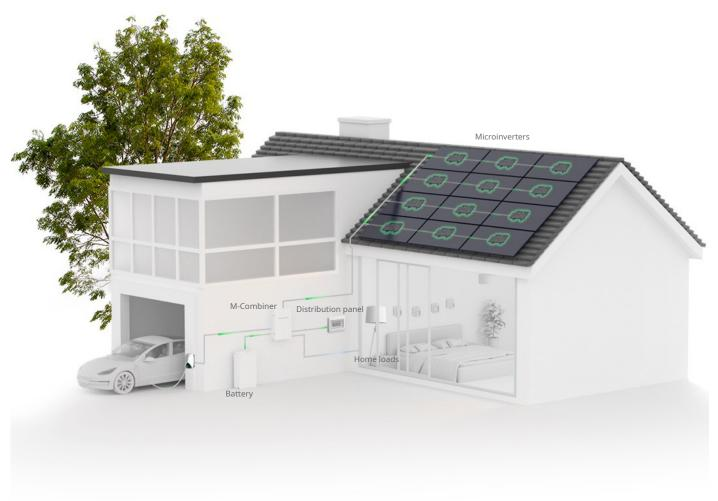
a. The battery nominal output power will be limited to 11.5 kW due to the 63A rated circuit breaker inside the M-Combiner.
