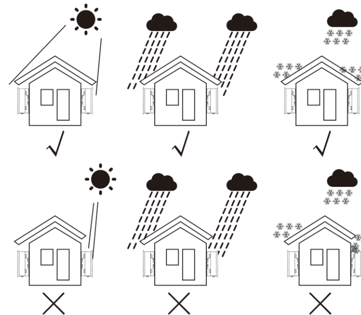
▲ Figure 4.1 Recommended Installation Locations
