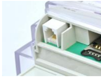
Figure 69: P1 port connection
