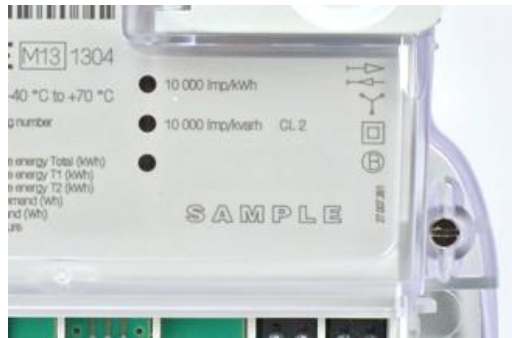
Figure 47: LEDs at MT382 meter
