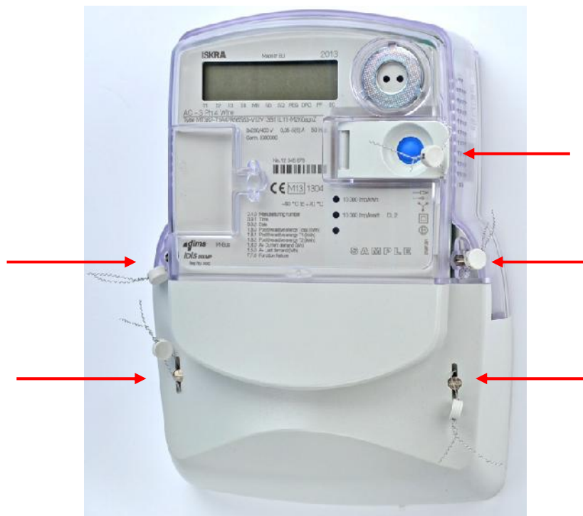
Figure 30: Positions of the seals at MT382 meter
