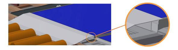
Add one top junction flashing between each top center flashing. Interlock those pieces together.
