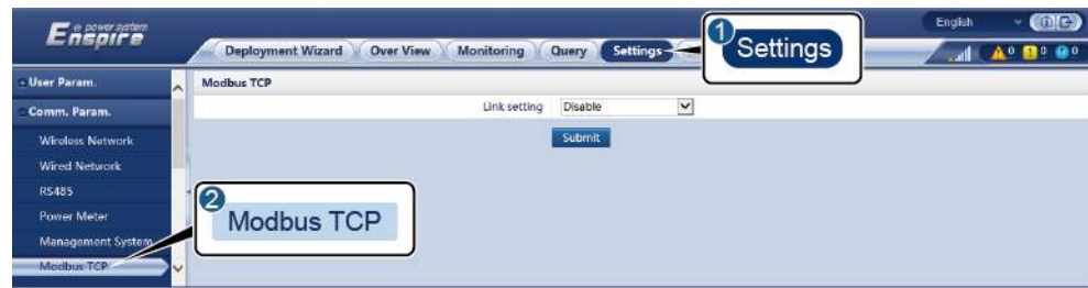
Figure 6-10 Setting Modbus TCP parameters
