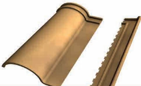
Tiles cutting for left flashing
