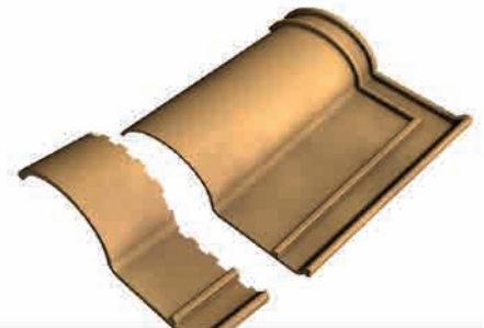
Tiles cutting for top flashing
