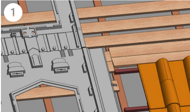
Installing the lateral flashing and tilt file
