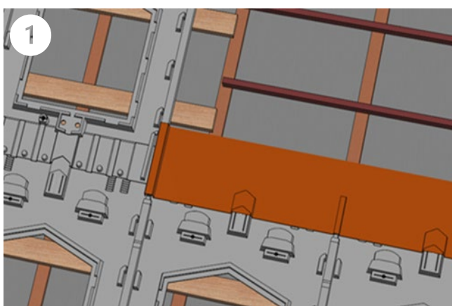
Installing the flexible waterproofing strip
