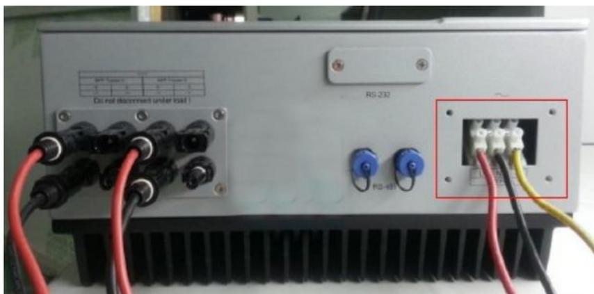
Fig.1 AC cables wiring
