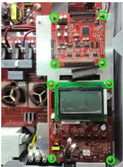
Fig.5.2.5 Screws on control board and COM board
