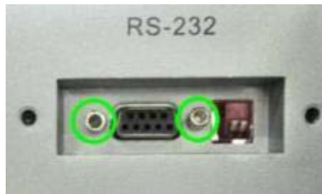
Fig.5.2.3 Two nuts on RS232 port
