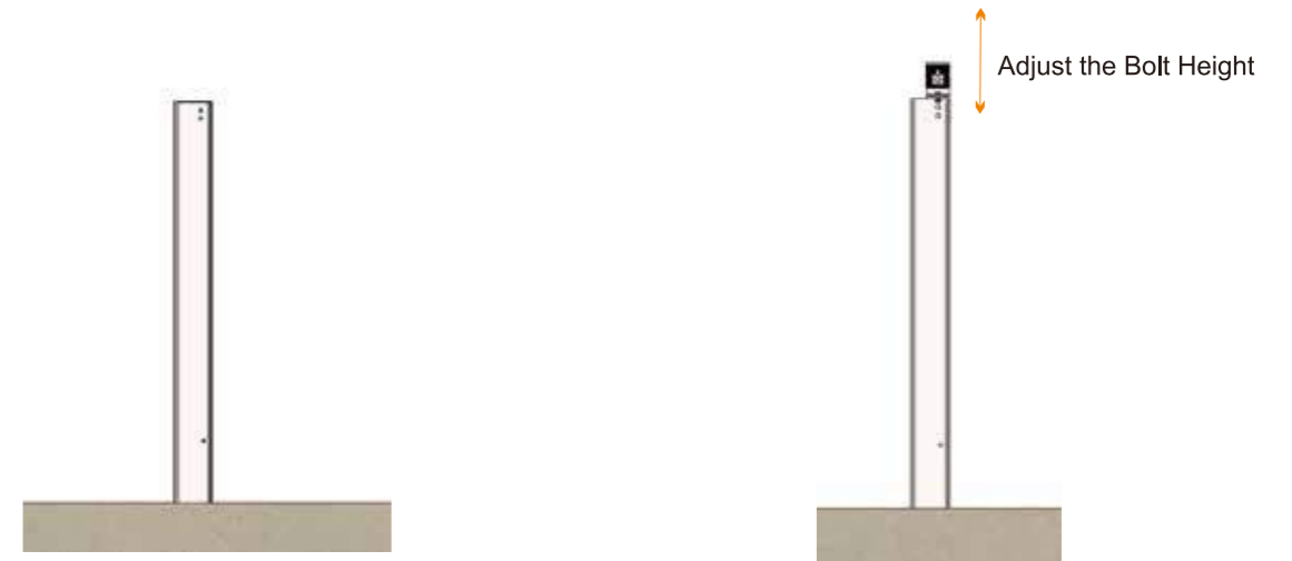
Step 1: Pile the Open Post by Pile Machine
