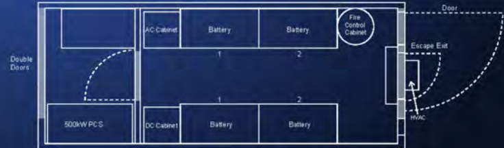
Standard 20' Container Solution 19.9×8.0×9.5 feet 100kW / 436kWh or 250kW / 763kWh
