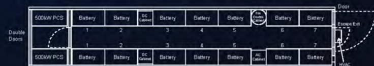
Standard 40' Container Solution 40×8.0×9.5 feet 1MW / 1MWh or 1MW / 2MWh
