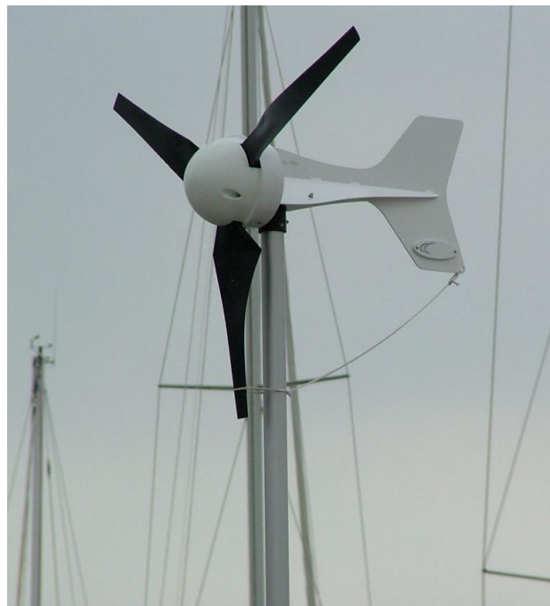
Fig-16: Tethering the rotor blades using the hole on the tail-fin (shown on an LE-300 Turbine)
