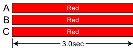
**Modbus Communication LEDs**
