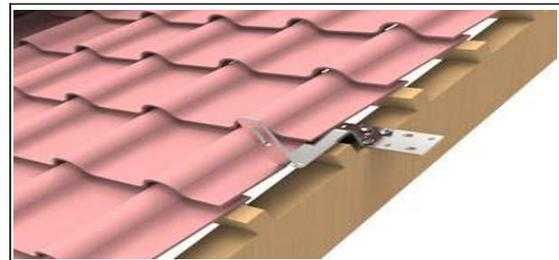
If necessary, use an angle grinder or hammer to cut a concavity in the tile that covers the roof hook at the point where the roof hook comes through. (Caution! Must not use fixed roof hook as a ladder, as this extreme point load could damage the tile below.
