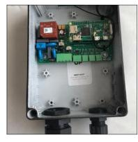
Clean out the EO Mini Pro 2 base for dust and attach the EO Mini Pro 2 base to the wall using four screws. Ensure that the base is the correct way up and that it is flush against the wall.
