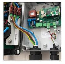
Connect the power cable to the front of the EO Mini Pro 2.
