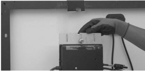
2. Thread the cap bolt into the threaded insert on the bracket, then slide middle channel of the microinverter onto the bolt.
