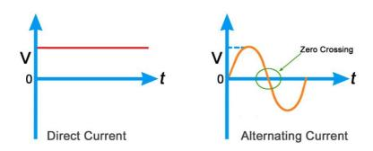
Figure 1: Representation of DC and AC
