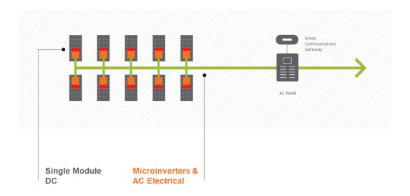
Figure 3: Representation of Enphase Microinverter system
