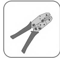
Crimping tool (10mm 2 , cold-pressed terminal)
