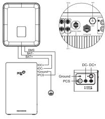
Note: Power Cable (K2) must be pulled straight from the battery DC+/- for more than 80mm before bending.
