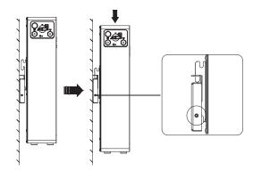
Insert 2 pcs of M5×10 screws (F2) into the holes on the left and right sides of the mounting bracket then tighten the screws.
