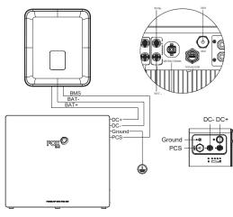
Note: Power Cable (K2) must be pulled straight from the battery DC+/- for more than 80mm before bending.
