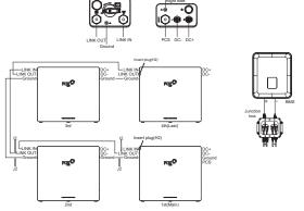
The steps for parallel connection of batteries are as follows:
