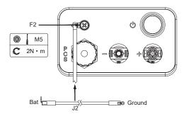
**b.** Connect the PCS Communication Cable (I2) of the **Main** battery to the BMS communication port of the inverter.
