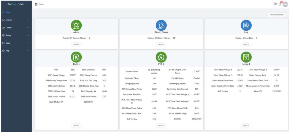
This page has a section for each of the device's setup and connected to the EMS, the number of sections displayed will vary depending on the current quantity of Meter, PCS and BMS setup.
