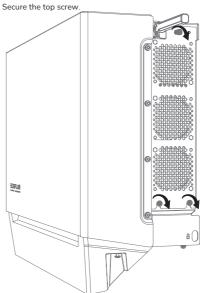
Secure the bottom screws, and lower the handle.
