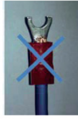
Terminal has been cut.
