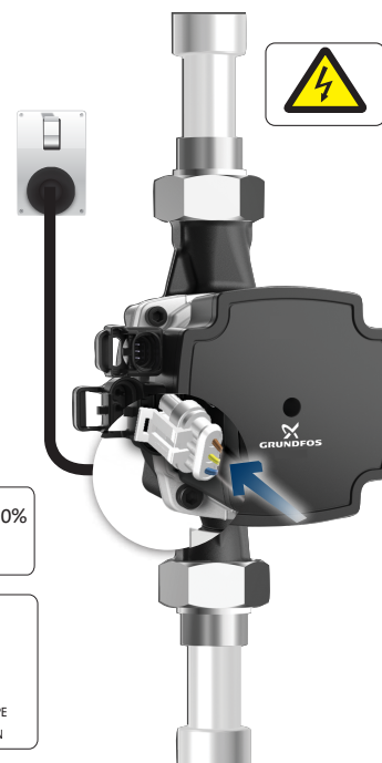
Control box without signal connection
