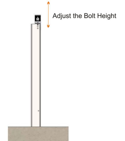
Step 2: Install and adjust the Top Cap
