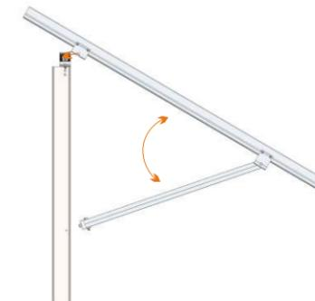
Step 3: Install the Assembly of Beam
