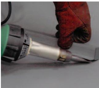
EJObar can be easily hot welded to make a very strong fix
