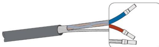
Figure 3-17 Crimping the communication cable
