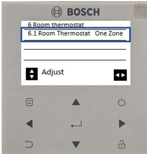
Press **Up** or **Down** Arrow to change the thermostat configuration.
