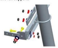
Step6 - attaching the bucket to the pole, after fixed the angle, tight all bolts
