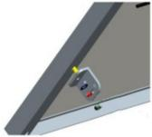
Step 2 - attaching 4 pcs Clips-A to the Bucket, and tighten the bolts
