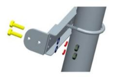
Step 3 - attaching the top Clips-B to the Clips-A
