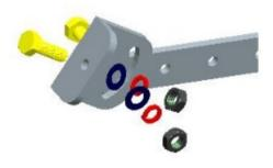
Step5 - attaching the bottom Clips-A to the two rail supports
