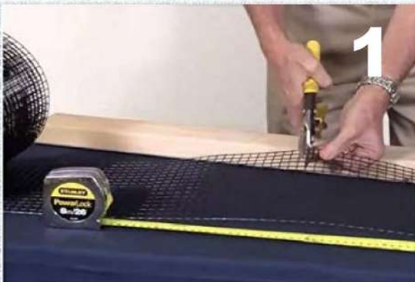
(1) Cut the PVC-coated mesh to an appropriate size for your solar panel.
